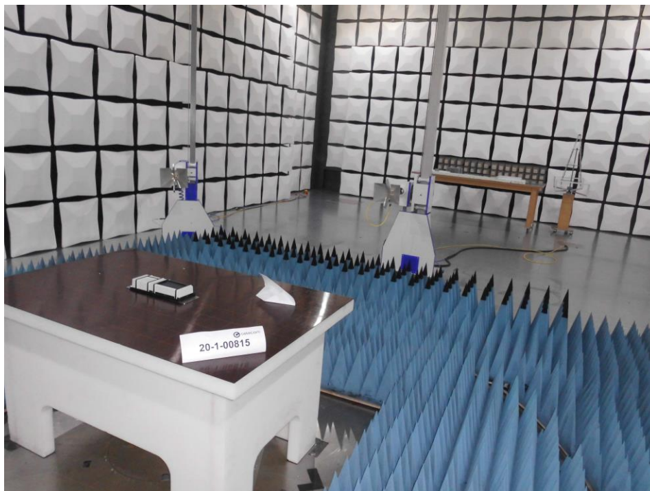
Picture 5: Test setup RF fields Immunity Test 5.1 – 6 GHz (setup rear side view – test with 3 V/m)
